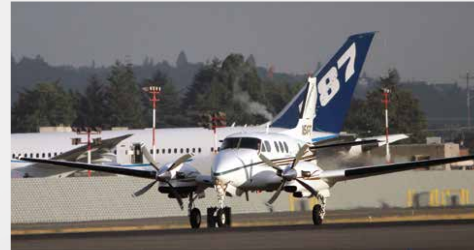
Swept Blade Propeller test airplane lands at Boeing Field
