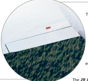
The trailing edge of the flaps have been recontoured and reshaped. The chord has also been extended. This component of ZR Technology has been incorporated to drastically reduce the wave drag that exists in the surrounding area of the aircraft.
