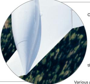
Of particular interest is the incorporation of ZR technology in the design of a uniquely effective Outboard Wing Trailing Edge Horizontal Winglet, or "Batwing." The Horizontal Winglet allows a reduction of the strong wing-tip vortices shed from the basic Learjet 35/36 wingtip-tanks.
