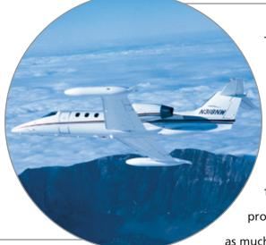
The overall airplane drag is substantially reduced. Certification flight tests have shown an overall cruise drag reduction of up to ten (10) percent or more at high speed. Drag reduction shows itself in all phases of flight, from takeoff, climb, cruise and letdown. Increased initial cruise altitude, faster cruise speed, longer range and reduced block fuel consumption are the resulting benefits.
