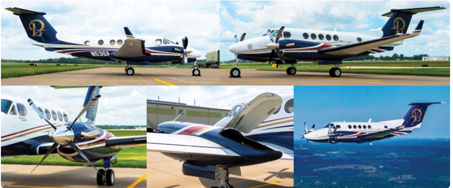
Top row, left to right: Side views show Raisbeck's Dual Aft Body Strakes, High Flotation Gear Doors, Crown Wing Lockers and Swept Props. Bottom row: 1) Swept Blade Propellers, 2) Crown Wing Lockers and High Flotation Gear Doors, and 3) test flight prior to delivery.
